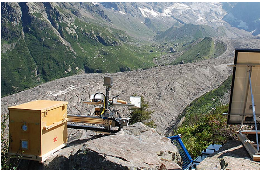
Fig. 2. The radar instrumentation and part of the power supply.
