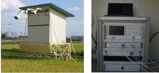
Fig. 1. Photos of an automatic scatterometer system: (left photo) The system was installed in a shelter with L, X and C-band antennas (from left to right) looking down the rice paddy field at 40° incidence angle; (right photo) The RF system inside the shelter is composed of a notebook computer, a vector network analyzer, a microwave switch, power unit, and an air conditioner.
