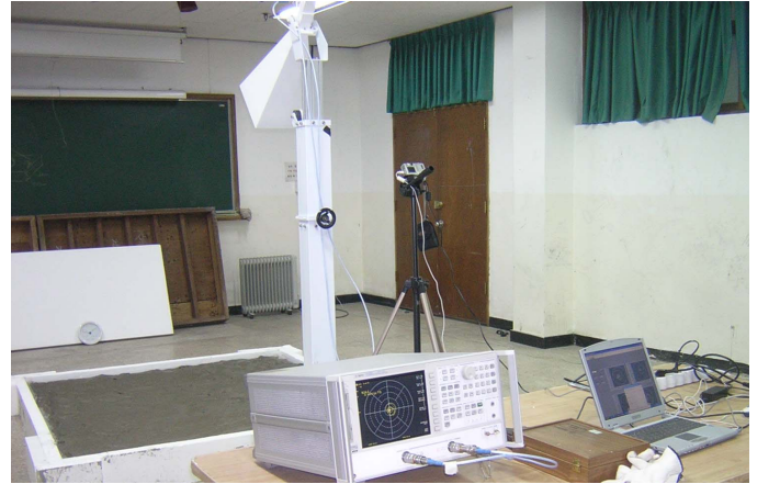
Figure 3. Photo of PolScat laboratory experiment on drying mud. The notebook computer automatically controls the the Agilent 8753ES network analyzer and the digital camera. This temperature controlled room was secured for 6 weeks.
