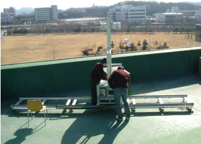
Fig. 1. GB-SAR system and field view of test site.
