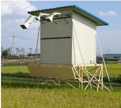
Fig. 1. View of L, C, X-band automatic scatterometer system.
