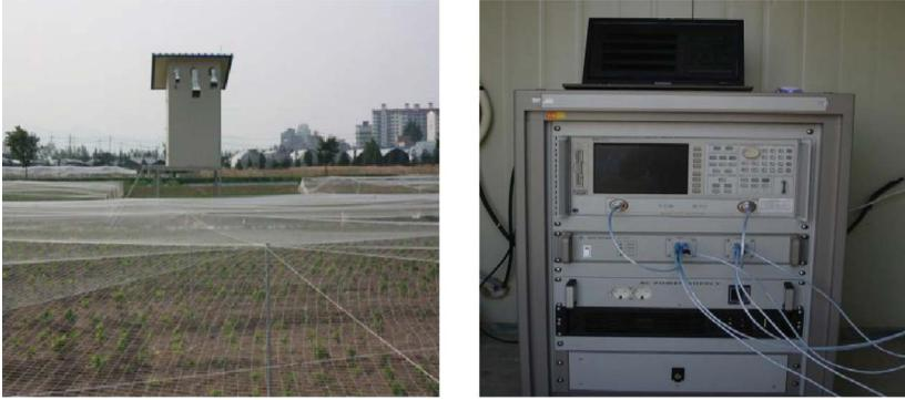
Figure 1. Photographs of the automatic scatterometer system. The system was installed in a shelter with the X-, L-, and C-band antennas (from left to right) looking down the soybean field at  $40^\circ$  incidence angle (left). The RF system inside the shelter is composed of a notebook computer, a vector network analyser, a microwave switch, power unit, and an air conditioner (not shown here) (right).
