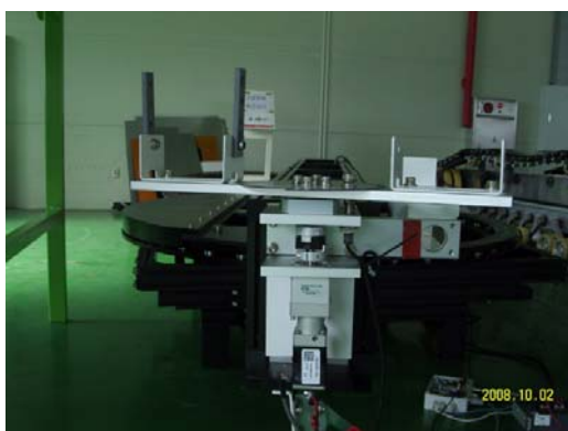
Fig. 4. Rotation motor for changing of a directivity of microwave radiation
