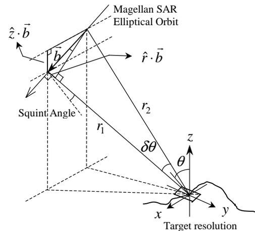
Fig. 1. Geometry of the sub-aperture interferometry (SAI) for Magellan satellite's elliptical orbit.
