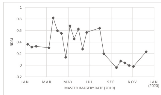
Fig. 9. Activity change of tailings piles in 2019 using NDAI graph. The reference point is the cyan pixel in the center of the expanded site shown in Fig. 8.
