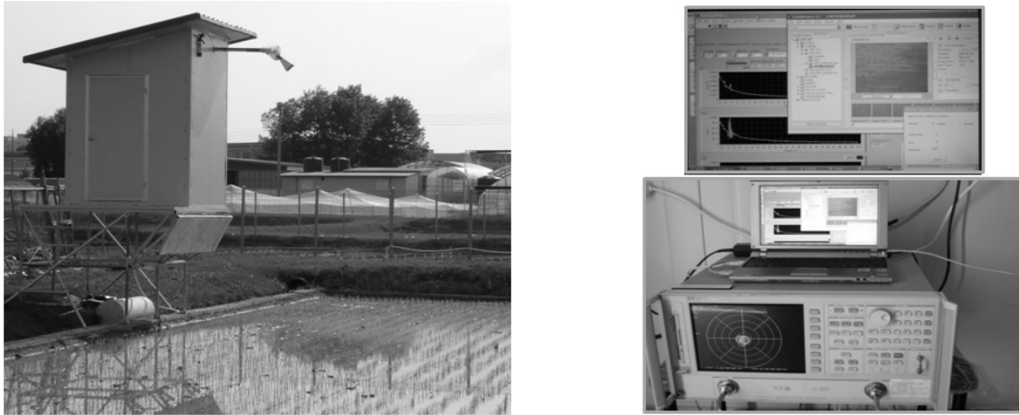
Fig. 1. Field view X-band automatic scatterometer system ; (left) The Shelter installed in the experimental paddy field with an X-band looking at the 45 degree ; (right) RF systems inside the shelter with network analyzer, RF cable and a computer that controls frequency, polarization and data storage.
