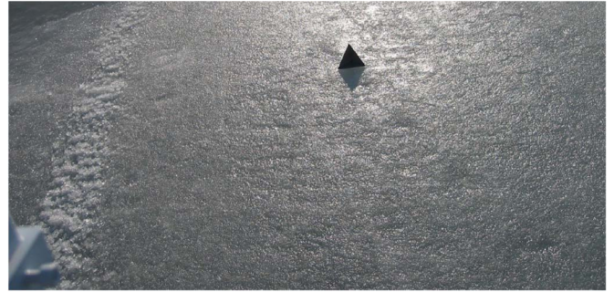
Fig. 1. Photograph of ice surface at the experiment site. The ice surface was clear of snow. A trihedral corner reflector on ice surface was used to calibrate the system.
