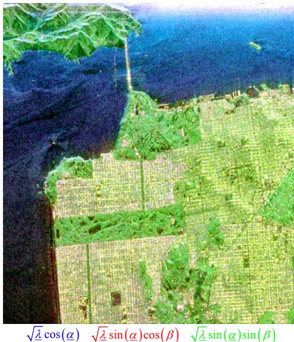
Figure 10 Main scattering mechanism provided by the eigenvector-eigenvalue based decomposition..
