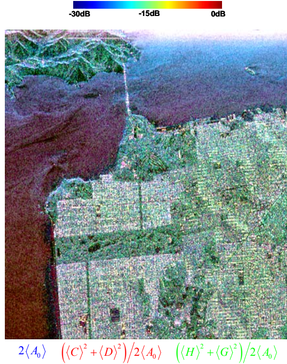
Figure 8 Elements of the parameterization of the coherency matrix provided by the Huynen decomposition.
