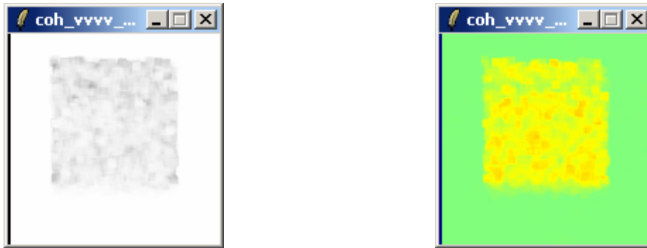
Figure 17 : Coherence images using an 11x11 window Amplitude (left) and phase (right)
