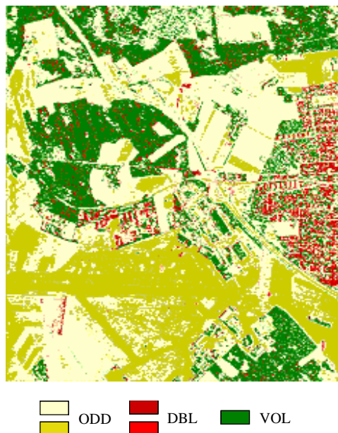
Fig. 28: Selection of significant mechanisms and identification to canonical scattering mechanisms (ODD: Single Bounce Scattering, DBL: Double Bounce Scattering, VOL: Volume Diffusion)
